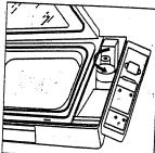
4. Replace with the new air filter, with *flow arrow* pointing down, turn filter clockwise.
