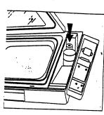
3. Remove air filter. Turn the air filter counter clockwise, lift up and remove.
